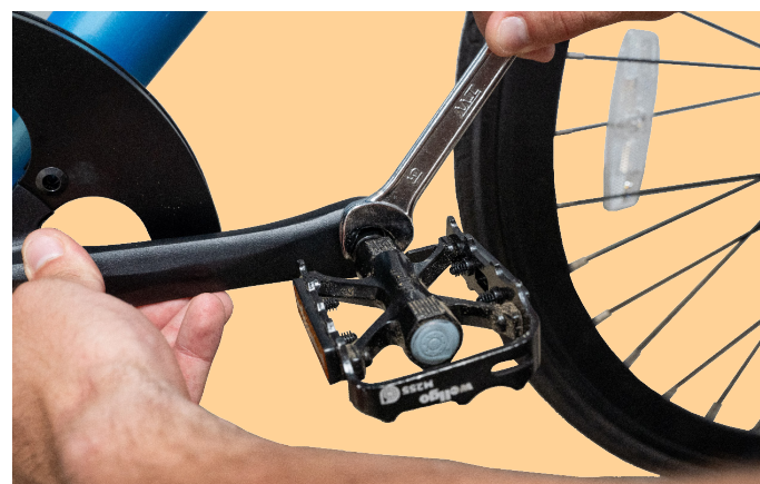
Figure 11. Attaching Pedal to Crank
