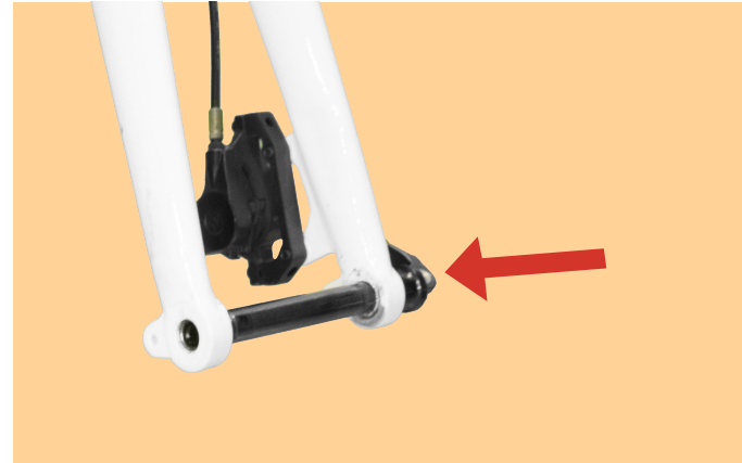
Figure 4. Locating Thru Axle Between Forks
