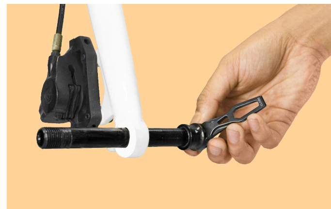
Figure 6. Removing Thru Axle from Forks
