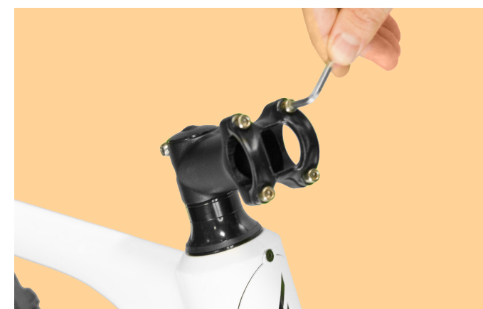
Figure 1. Stem Plate Bolt Removal
