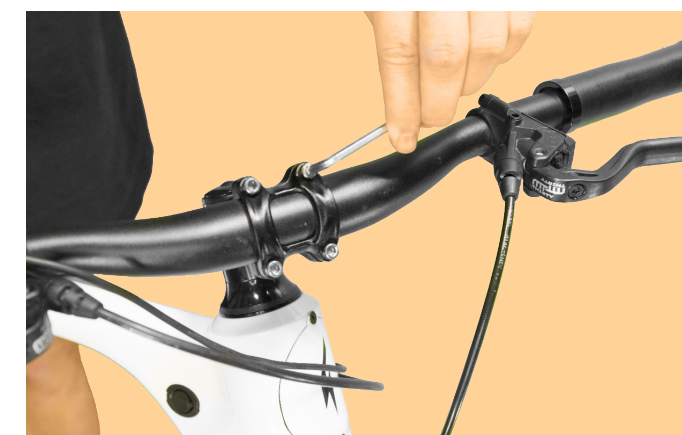
Figure 2. Tightening Stem Plate Bolts
