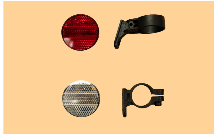
Figure 15. Rear and Front Reflectors
