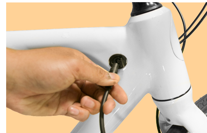
Figure 18. Charging Your Battery
