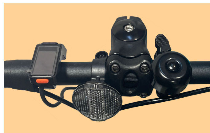
Figure 17. Bell and Reflector Setup on Handlebars
