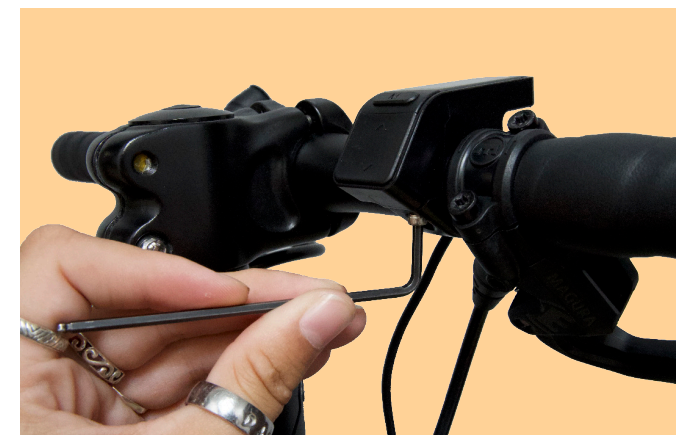
Figure 13. Tightening the LDC Display
