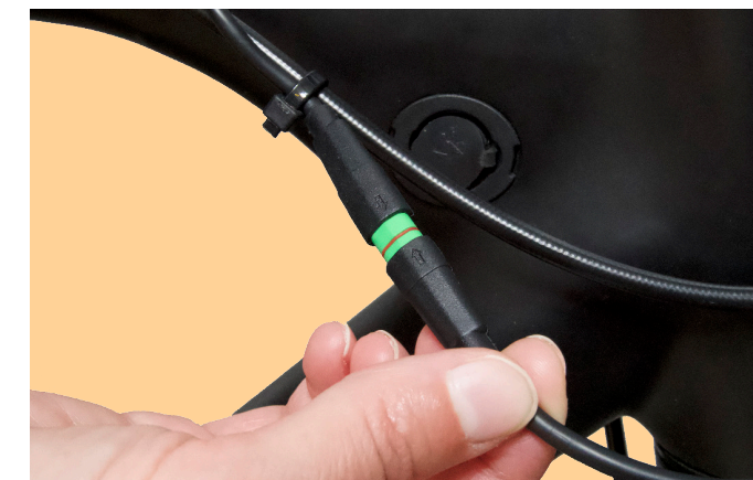
Figure 14. Connecting the LCD cables
