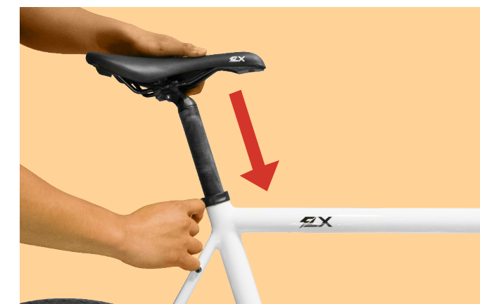
Figure 12. Dropping Seat Post into Seat Tube
