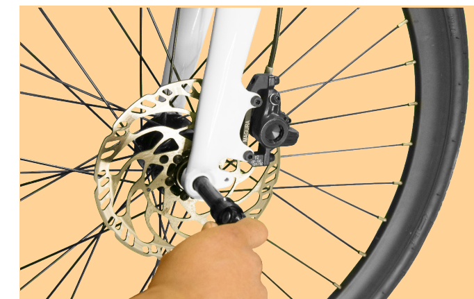
Figure 8. Inserting the Thru Axle
