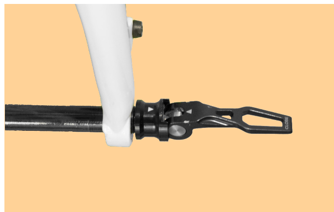
Figure 5. Opening Cam Lock Lever
