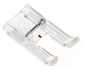
This foot provides an unobstructed view of your work while sewing since there is no bridge between the toes. In addition, there is a groove on the underside to allow dense decorative stitches to pass underneath without jamming. Both of these characteristics make this foot ideal for doing **applique**. Great for decorative work and showing of those special stitches on your sewing machine as borders for cushion covers, table linens and more.
