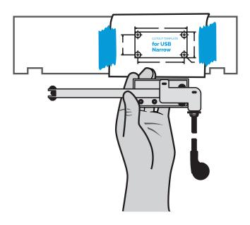
**Step 4 -** With a 1/2" drill bit, drill a hole in each corner, being careful not to splinter the wood on the inside of the drawer box. Using one of the 1/2" holes, insert a jigsaw and then make the required cutouts in the drawer box.
