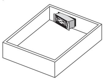
**Step 6 -** Align arms. With the drawer mostly closed, mark the position of the rear mounting bracket. It is important to make sure the drawer moves freely in and out and that the arms are square and even. Spend sufficient time at this step before fastening the bracket to the rear wall to make sure everything is square and the arms are in the correct position. Once that is done, secure with the screws provided.
