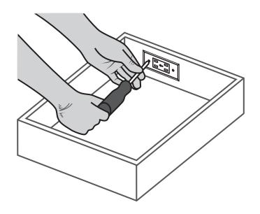
**Step 8 -** Connect the Docking Drawer power cord to the in-cabinet electrical supply. For more details about locating an in-cabinet electrical supply for your Docking Drawer installation, please refer to the Electrical Planning Guide located in the Specification Library at www.dockingdrawer.com.
