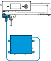
The Safety Interlock Box uses a limit switch to de-energize the outlet when the drawer starts to close and can be added to any 15 or 20 amp Blade Series outlet. The Safety Interlock Box is optional in the US and can be added as a second layer of safety for additional peace of mind. In Canada, the Safety Interlock Box satisfies the requirements of the Canadian Electrical Code (CEC) for AC outlets in enclosed spaces.
