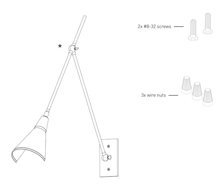
\* Please note that the Magari is used here as an example in order to illustrate how to install fixtures that don't include a mounting plate. This style of fixture is installed directly into a junction box. For a full list of such fixtures, please refer to the Installation Instructions page on our website.
