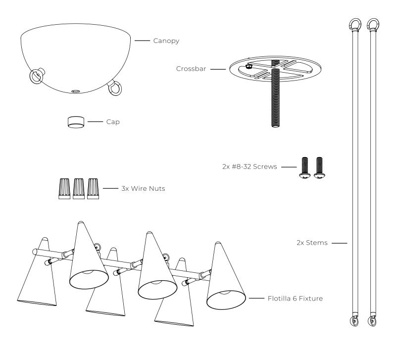
1. Mount the crossbar-nipple assembly to the junction box using the provided #8-32 screws.
