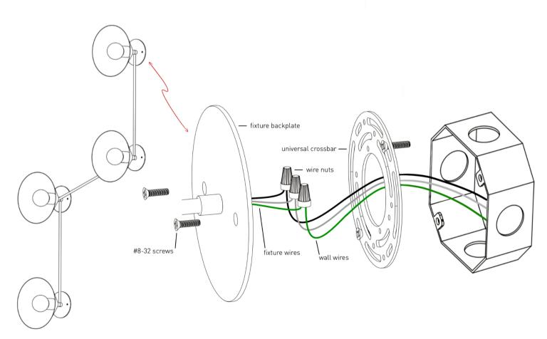
8. Mount the remaining 3 backplates to the wall by screwing x6 of the provided  $\#8 - 32 \times 11/2$  screws into the drywall anchors.
