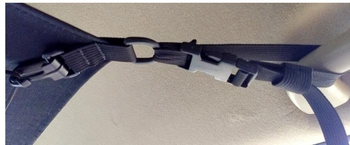
Figure 2. A corner attachment strap clipped around one of the interior grab handles. Note that the plastic buckle to the right of the D-ring is facing downward. This is the correct orientation.
