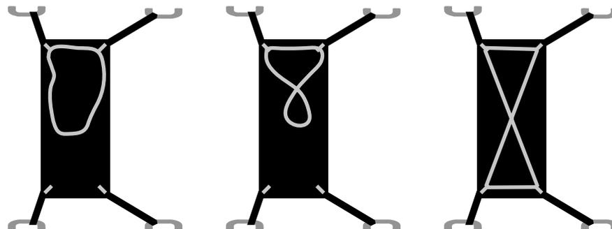
Figure 4. To attach the elastic retention cords, take one of the cords and clip it into two of the corner clips on one side of the bottom of the Cargo Hammock (as shown in the first image above). Twist the cord (as shown in the second image) and clip the resulting loop into the third and fourth corner clips (as shown in the third image above). You can adjust the tension of the cords by pulling the ends through the toggle.
