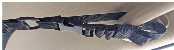
Figure 3. The excess webbing on a corner attachment strap looped back onto itself several times and tucked into the elastic retaining loop.
