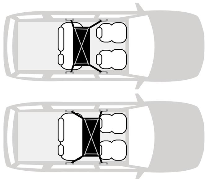
Figure 1. The upper image shows how most people will want to configure their Cargo Hammock (with the longer straps clipped around the front pair of grab handles). The lower image shows the Cargo Hammock reversed, which is an alternate choice that may or may not work better for you.
