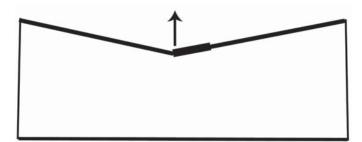
3. Connect bars by releasing the spring-loaded cap. Repeat same process for the other side of the crate.
