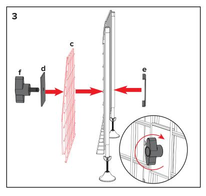
Use parts (d), (e), and (f) to secure the side segments (c) to the main segment (a). Test to make sure the barrier is securely in place.
