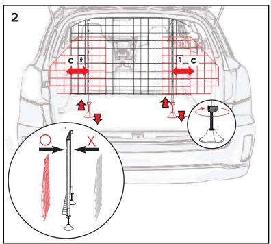
Place the largest piece of the barrier (a) in the center of your cargo space with the flat surface against the back seat. Make sure the top of the barrier contacts the ceiling of your vehicle.
