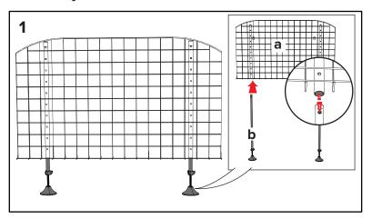
Slide legs (b) into the largest piece of the mesh barrier (a) on left and right sides.
