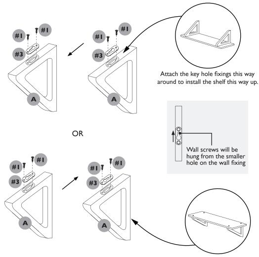
Attach the key hole fixings this way around to install the shelf this way up.
