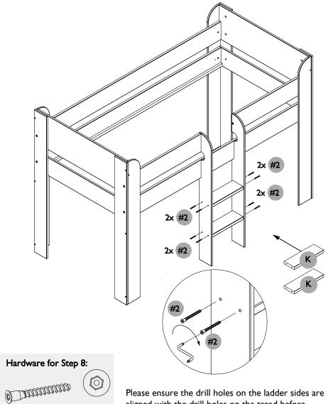
Please ensure the drill holes on the ladder sides are aligned with the drill holes on the tread before inserting & tightening hardware (#3)with the allen key.
