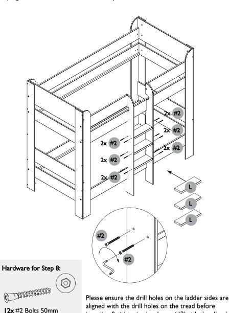
inserting & tightening hardware (#2)with the allen key.
