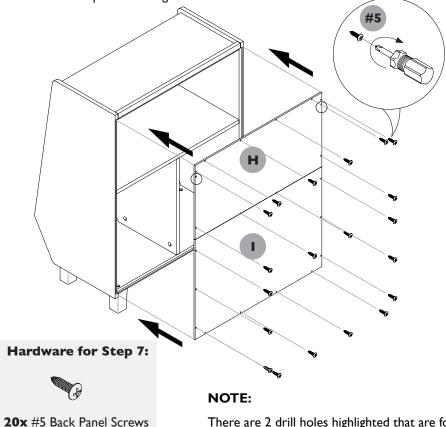
There are 2 drill holes highlighted that are for attaching the anti-tip kit brackets. Please use the anti-tip kit provided to tether your unit to the wall for safety.
