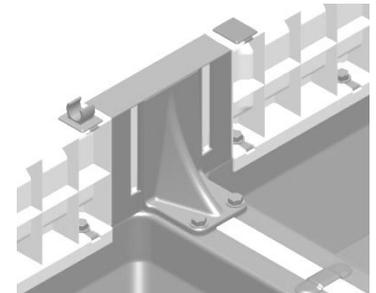
6. Push **short** bolts into all of the holes that join the top rim panels to the base containers. Push **long** bolts into the holes in the support braces.
