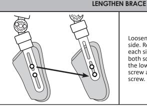
Loosen screw in **bottom slot** on each side. Remove screw in top slot on each side. Slide hinge vertically so both screw holes on each side are in the lower slot. Re-tighten the loose screw and re-insert/tighten the other screw. Repeat on the other side.
