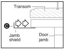
As always when drilling around glass, make sure the drilling and screw placement will not contact the casement of the glass enclosure.
