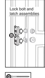
**3.** With the Door Shields in place, make sure the Door Shields are level and flush against the door slab on all sides.
