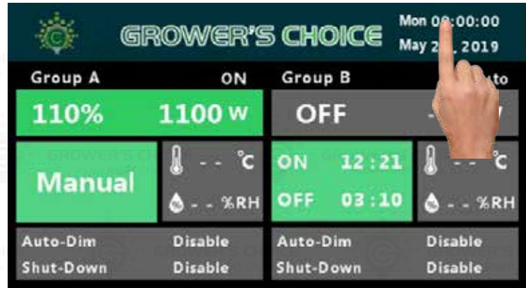
Touch the date and time for access to the controller clock calendar
