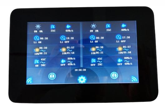
The wired control system was developed by RS485 bus communication protocol. It's mainly composed of the main controller and RS485 adapter board. We also developed the temperature and humidity meter accessories for people easy to check the growing environment.
