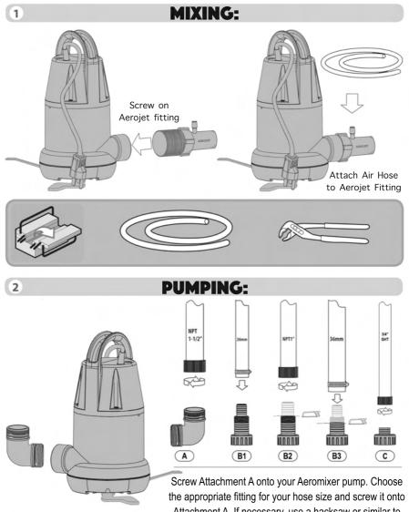
Attachment A. If necessary, use a hacksaw or similar to modify Attachment B as pictured. Secure using hose clamp.
