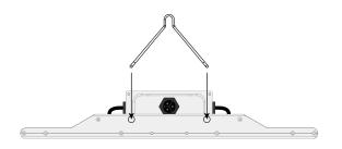
2 • Use ratchet hangers to lift Fixture into place.
