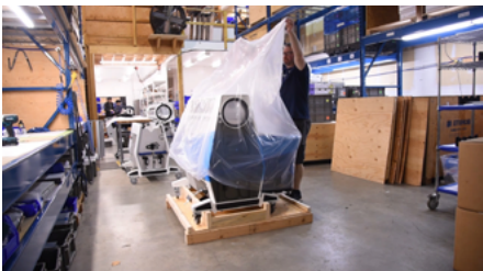
4. Remove protective plastic from M108S and retain for future use
