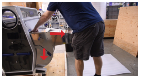
9. Push down 'hockey stick' lever to unlock the separator and slide the separator out until a hand-sized gap is visible
