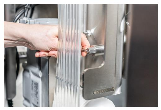
Move to the back side of the Sorter and open the tailgate by releasing the two compression latches.
