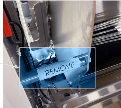
4 If the supports aren't removed, the operator will not be able to disassemble the belts off for cleaning.
