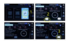
STEP 2: Check the printed model. Find the alignment line in X and Y direction and set the corresponding offset X and Y values, press "OK".
