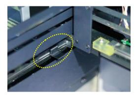
STEP 4: Pull the buckle upward and take away the stop block on the right linear guide.
