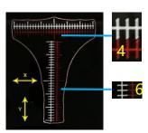
If there are no lines are aligned with each other, set 15 firstly on the corresponding direction ("+/-"), redo the printing and reset the offset value.
