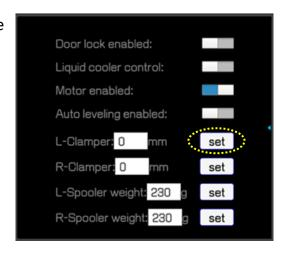
STEP 4: Click the "←" icon to let the two gears closer and closer. Insert and draw out the calibration steel bar after every screen click until you feel the resistance from the gears. After that click "Set" to save the value. The higher the value, the greater the clamping force.
