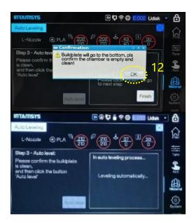
**STEP 8:** Press "Finish" after leveling is successful, the build plate will go downwards and then upwards to Z home.
