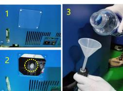
The volume of the liquid tank of the chiller is 1000ml, and the liquid level sensor will be triggered when it is lower than 600ml.
