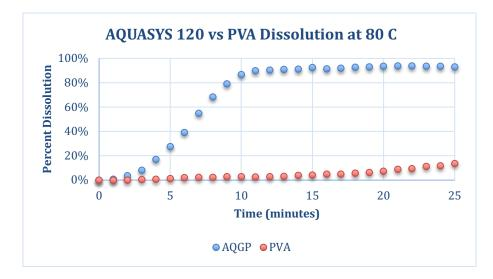
Figure 1. Dissolution Kinetics of AQUASYS 120 and PVA
