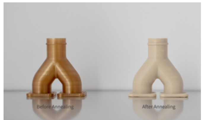
Figure 8: Manifold printed with VICTREX AM 200 filament, before and after annealing (Photo courtesy of Intamsys).
