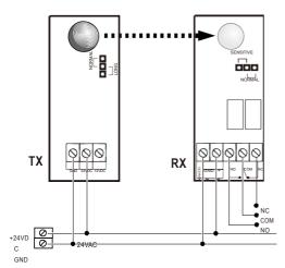
Figure 2. Connect with 24VDC or 24VAC
