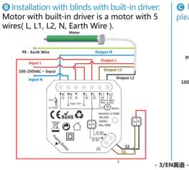
please refer to below wiring diagram. PE - Earth Wire Input L 100-250VAC ~ Input Input N Output L2
