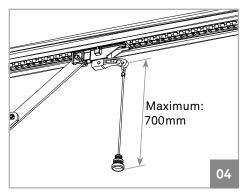
← Together with the automatism it is also provided a string to apply on the unlock lever, which makes it even a more practical and comfortable process.
