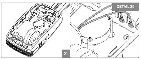
In case of automatism failure or malfunction, you must detect the fail component (motor or central). To do that, you should test the motor directly connected to a **24V DC** power source, in order to understand if this works.
