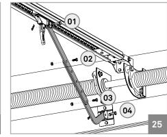
**07** • Now attach the two connecting rods between the trolley and the panel's upper plate.
