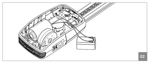
Motor cables have no specific way of connection. The only difference is that if you connect the motor in one way, it will rotate in one direction, and if you connect the wires in the oppose it will rotate in the other direction.
