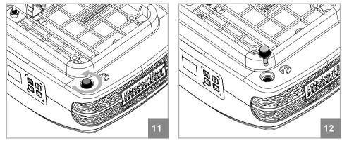
• To replace the fuse, first loosen it as visible in the image 11. Then just pull to remove it (image 12). Repeat the same steps in reverse order to put a new fuse. The operator uses a 250V 2,5A.
