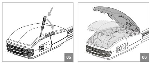
To remove the cover simply insert a small screwdriver into the side holes, and create a leverage effect to release the indents fittings between the top cover and the body. Then just remove the cover by lifting it.
