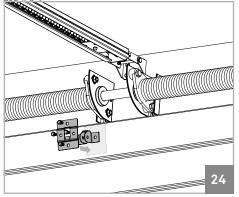
**06** • Attach the plates to the top of the door panel. The rods must be centered horizontally with the panel so that it stays aligned with the rail.
