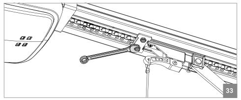
• To install the opening stopper just apply it on the rail, as seen in Figure 34. The stopper must have a metal plate out of the rail and other on the inside, so when you fasten it, this is secure in the pipeline.
