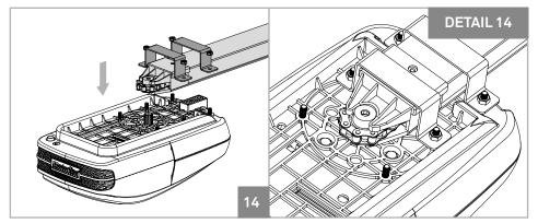
**02** • The aluminum rail and automatism attachment must be made using the plates and M6 nuts and as shown above. Tighten 4 screws, leaving the two in the front free.
