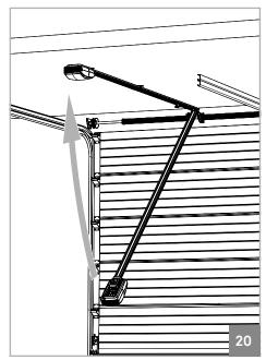
**04** • Raise up the motor until the rail is levelled horizontally.
