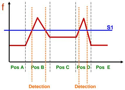
In this application, the sensitivity is adjusted via the potentiometer to the value \$1. This means that every frequency superior to this limit creates detection and therefore relay activation.
