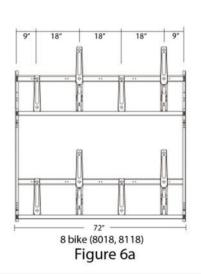
Note: For multiple units, assembly should be modified to continue staggered positions. Four additional bolt "I" and nut "M" are included to connected parts "A" and "B" for adjacent setups.
