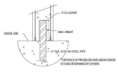
NOTE: THIS TYPE ANCHORING IS ALSO USED AS A BARRICADE. BOLLARD HELD IN PLACE BY STEEL PIPE STEEL PIPE MUST BE ANCHORED IN CONCRETE FOOTING TYP. 12" DIA. CONCRETE BOLLARD SAME ANCHORING SYSTEM USED ON14" AND 18" DIA. OR SQ. BOLLARDS
