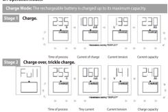
Discharge Mode: It is used to reduce the memory effect. The rechargeable battery is discharged to a preset battery voltage (0.9v). Once discharge is finished, the battery will be charged at the pre-selected charging current. Discharge current is always half of the selected charge current.
