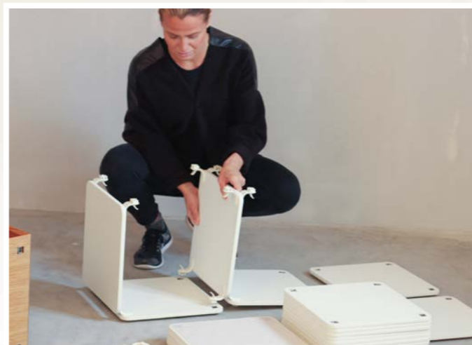
14. Slide the newly assembled panels towards the structure, and attach to the first base panel.
