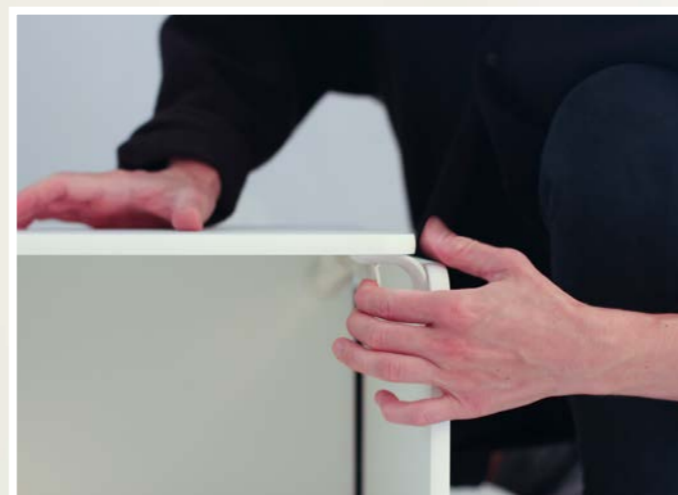
24. Lock the top panel in place. Make sure there is no gap between connectors and panel.
