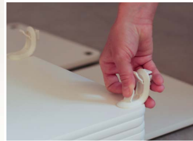
5. Make sure there is no gap between connector and panel before you engage the lock by pressing down the lever.
