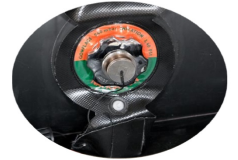
Intercommunication / Inflation Valves Safety / Inflation
