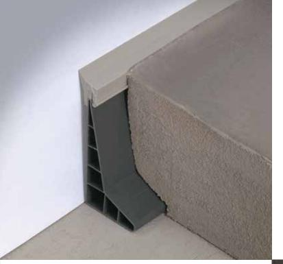
Expansion joints around the perimeter of the floor layout provide concrete with the necessary gap for differential movement. **JOINTEC GC** profiles coupled with the GCP and GCR synthetic inserts in soft Resilflex allow the concrete to be poured, leveled and cured in one simple step, while still accommodating its expansion and contraction. The perimeter joint eliminates the need for base boarding.
