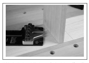
With the holes drilled, test fit the joint. (See Figure #30)
