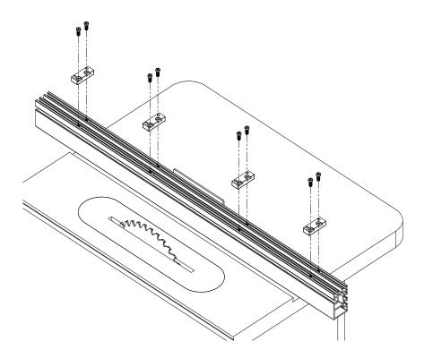
Slide the 8 square nuts into the T-Tracks on your Unifence Fence. Position the mounting blocks over the square nuts and inserts 8 of the 1/4"-20 x1/2" LHCS into the sunken openings on the mounting blocks (see image above). Once the screws are in place, line up the Track with the blocks before tightening.
