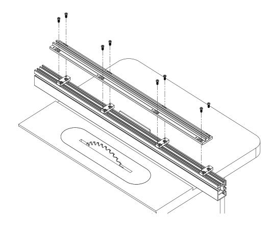
Once the mounting blocks are securely in place, position the track over the tapped holes on the mounting blocks and insert the remaining (8) 1/4"-20x1/2" LHCS (See image above). Tighten!!
