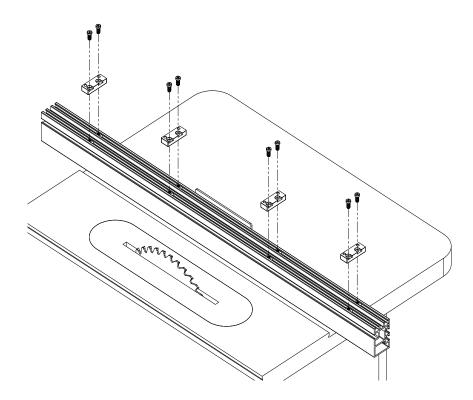
Slide the 8 square nuts into the T-Tracks on your Incra Fence. Position the mounting blocks over the square nuts and inserts 8 of the 1/4"-20 x1/2" LHCS into the sunken openings on the mounting blocks (see image above). Once the screws are in place, line up the Track with the blocks before tightening.
