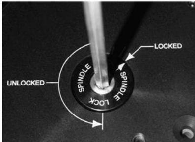
To lock your lift turn lift handle clockwise to the "LOCKED" position
