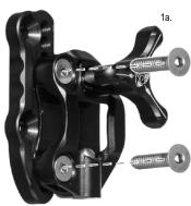
Mount Compound or Recurve Plate to bow riser with screws provided (1a.). Tighten mounting screws securely.
