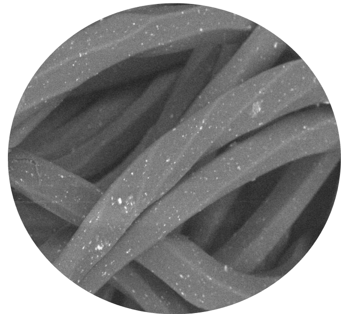
Ionic silver atoms permanently extruded in the fiber or filament.
