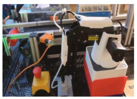
DOBOT Magician adapts to Siemens PLC system, which is used by Volkswagen for its teaching production line.
