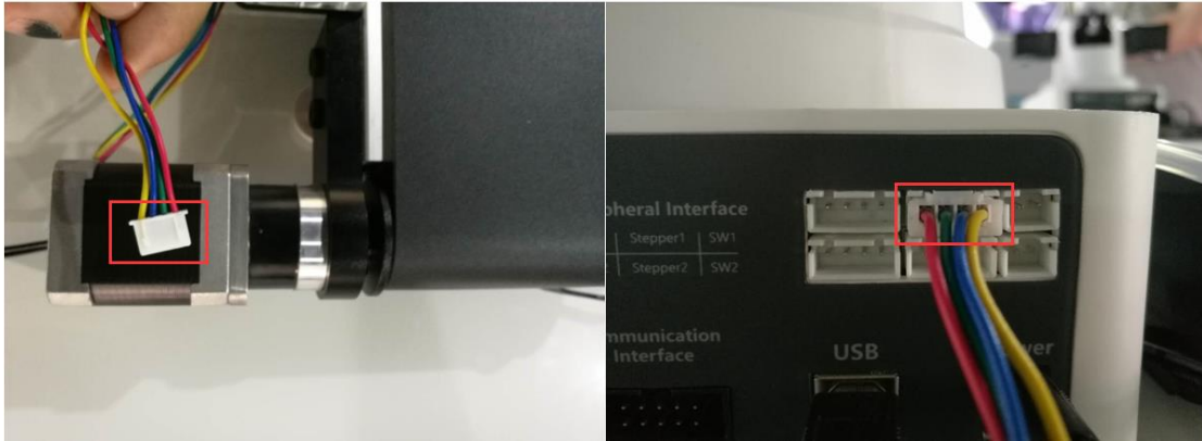
Figure 1.4 Connecting the motor wire
