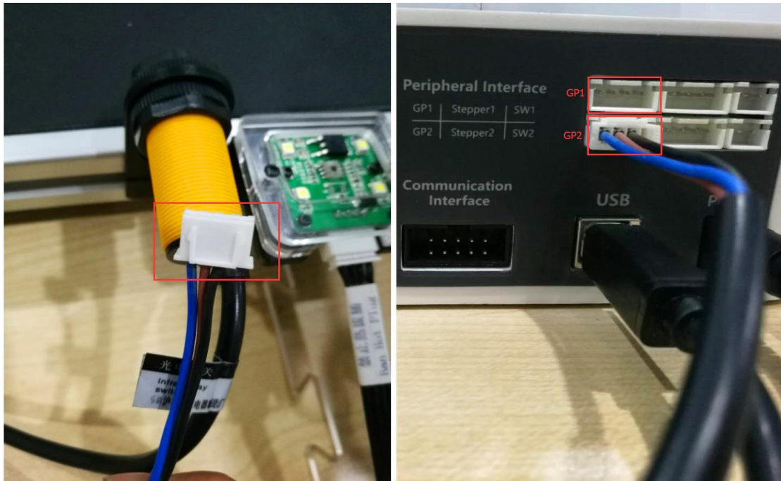
Figure 1.6 The photoelectric sensor connection
