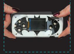
Place one of the button caps at each of the six dots indicating where the pushbuttons should be (left, right, up, down, A, and B). Don't worry if the pushbuttons look a bit tilted. They'll stay in place once the second casing is placed on top of them.
