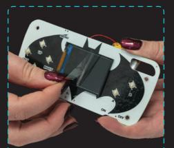
We can remove the protective foil from the display now that it is secure.
