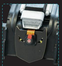
Stick the camera between the "eyes" of the Batmobile™ in the middle of the headboard. Make sure the headboard is connected to the "Front LED" port. It's time to take the fire board with red LEDs.
