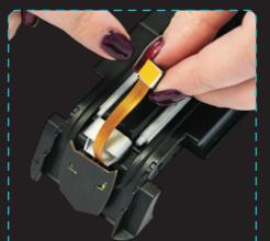
After you've tightened the headboard, you can attach the camera to it.
