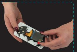
Make sure the display is on the correct side and that the ribbon is pulled through the correct hole.
