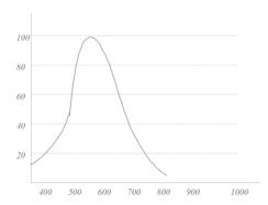
$Wave length \ \lambda \ (nm)$  Spectrum Response Characteristic
