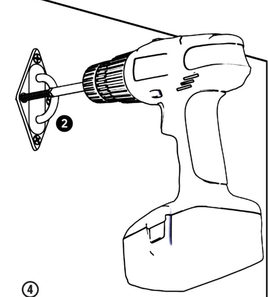
Insert the screw into the plastic anchor to fix the padeye
