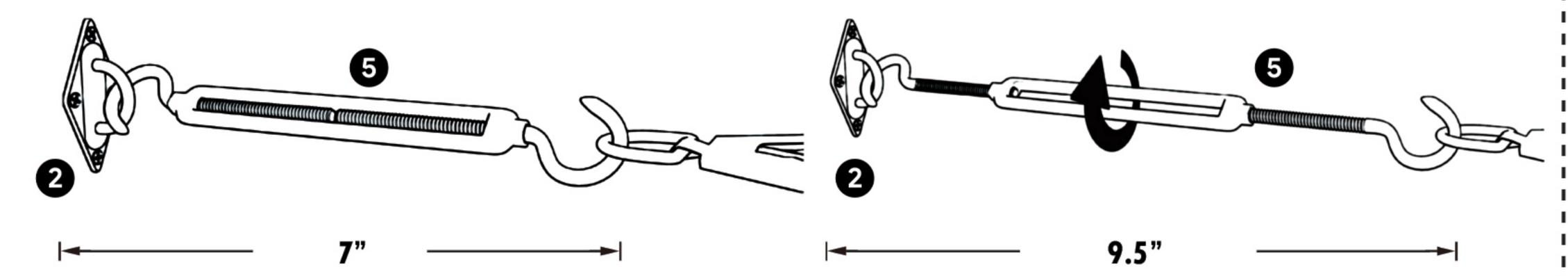
Turnbuckle Can Be Extended 7" to 9.5"
