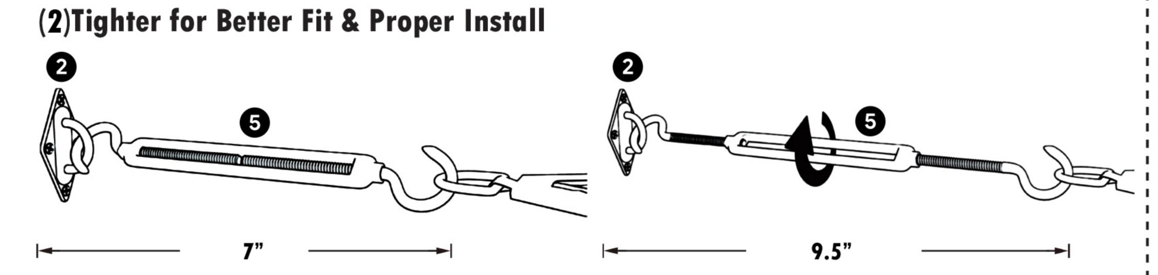
Turnbuckle Can Be Extended 7" to 9.5"
