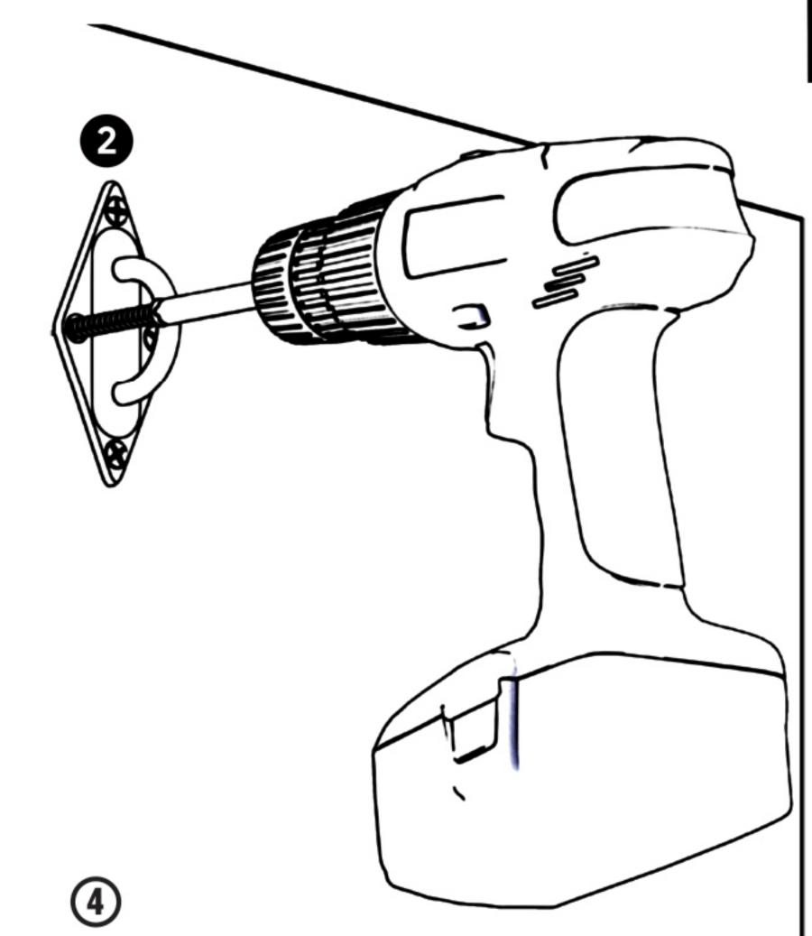
Insert the screw into the plastic anchor to fix the padeye
