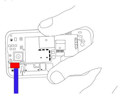
Using a safe open pry tool, remove the rubber on top of the motherboard. Disconnect the two pop connectors to separate the motherboard. Remove the motherboard
