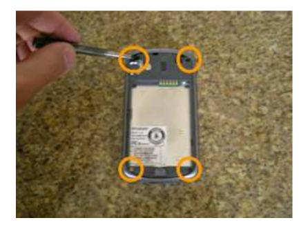
Remove the 4 screws as shown in the picture above using the T6 screwdriver.
